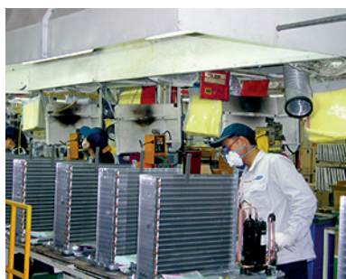
Outdoor units production
